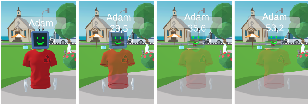
Figure 4.16: Collaborator becoming gradually more transparent as their temporal distance to the user increases. For this visualisation the reference user was temporally positioned at 27.9 seconds on the time slider. The label of the collaborator shows their temporal position by the numeric value below their nametag as soon as the users do not reside at the same point in time.
