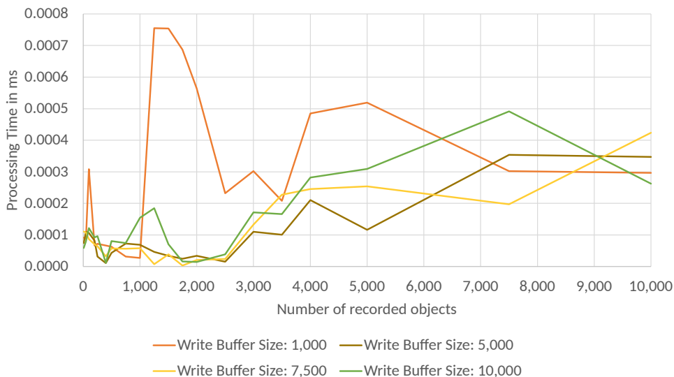
Figure 3.3: Average time required to record transformation data of a single object for a given point in time across different write buffer sizes.
